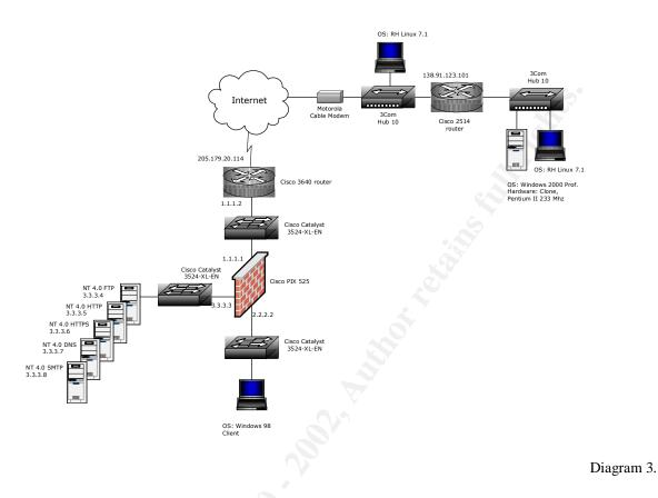
Among the resources used by the red team are a Cisco 2514 (dual-ethernet) router, hubs, Internet access through a cable modem, a Windows 2000 Professional workstation and a Red Hat Linux workstation. All of these resources are readily available at little cost.
